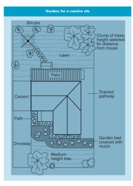
extend outwards a minimum of 900 mm (more in highly reactive soil) and should have a minimum fall away from the building of 1:60. The finished paving should be no less than 100 mm below brick vent bases.
